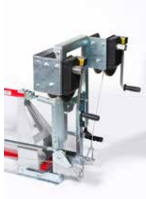
Extra third winch when using longer screeds to avoid bending in the middle
