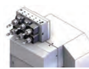
6 tools (Driven max. 5) ※ Tool distance : 50mm
