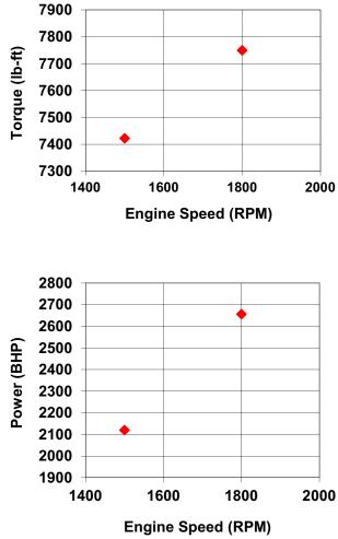
All data is based on the engine operating with a fuel system, water pump, lubricating oil pump, air cleaner, and alternator. The fan, optional equipment, and driven components are not included. Data is based on operation at SAE standard J1394 conditions of 300 ft. (91.4 m) altitude, 29.61 in. (752 mm) Hg dry barometer, and 77  $^\circ\text{F}$  (25  $^\circ\text{C}) intake air temperature, using No.2 diesel fuel only.$
