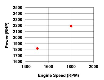
All data is based on the engine operating with a fuel system, water pump, lubricating oil pump, air cleaner, and alternator. The fan, optional equipment, and driven components are not included. Data is based on operation at SAE standard J1394 conditions of 300 ft. (91.4 m) altitude, 29.61 in. (752 mm) Hg dry barometer, and 77 °F (25 °C) intake air temperature, using No.2 diesel fuel only.
