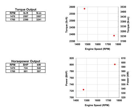
All data is based on the engine operating with a fuel system, water pump, lubricating oil pump, air cleaner, and alternator. The fan, optional equipment, and driven components are not included. Data is based on operation at SAE standard J1394 conditions of 300 ft. (91.4 m) altitude, 29.61 in. (752 mm) Hg dry barometer, and 77 °F (25 °C) intake air temperature, using No.2 diesel fuel only.
