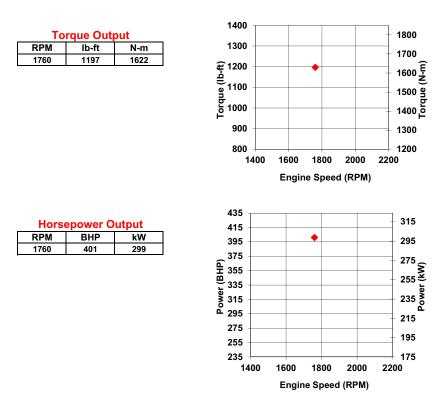
All data is based on the engine operating with a fuel system, water pump, lubricating oil pump, air cleaner, and alternator. The fan, optional equipment, and driven components are not included. Data is based on operation at SAE standard J1394 conditions of 300 ft. (91.4 m) altitude, 29.61 in. (752 mm) Hg dry barometer, and 77 °F (25 °C) intake air temperature, using No.2 diesel fuel only.
