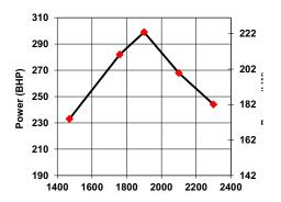
All data is based on the engine operating with a fuel system, water pump, lubricating oil pump, air cleaner, and alternator. The fan, optional equipment, and driven components are not included. Data is based on operation at SAE standard J1394 conditions of 300 ft. (91.4 m) altitude, 29.61 in. (752 mm) Hg dry barometer, and 77 °F (25 °C) intake air temperature, using No.2 diesel fuel only.
