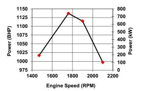
All data is based on the engine operating with a fuel system, water pump, lubricating oil pump, air cleaner, and alternator. The fan, optional equipment, and driven components are not included. Data is based on operation at SAE standard J1394 conditions of 300 ft. (91.4 m) altitude, 29.61 in. (752 mm) Hg dry barometer, and 77 °F (25 °C) intake air temperature, using No.2 diesel fuel only.
