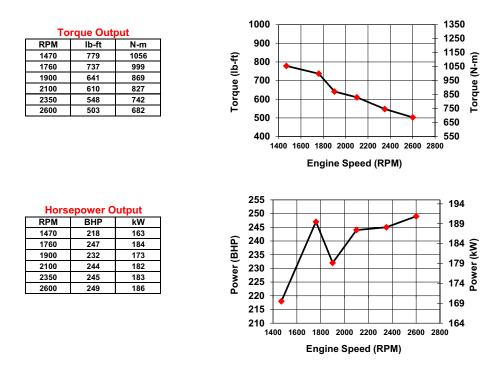
All data is based on the engine operating with a fuel system, water pump, lubricating oil pump, air cleaner, and alternator. The fan, optional equipment, and driven components are not included. Data is based on operation at SAE standard J1394 conditions of 300 ft. (91.4 m) altitude, 29.61 in. (752 mm) Hg dry barometer, and 77 °F (25 °C) intake air temperature, using No.2 diesel fuel only.
