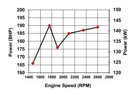
All data is based on the engine operating with a fuel system, water pump, lubricating oil pump, air cleaner, and alternator. The fan, optional equipment, and driven components are not included. Data is based on operation at SAE standard J1394 conditions of 300 ft. (91.4 m) altitude, 29.61 in. (752 mm) Hg dry barometer, and 77 °F (25 °C) intake air temperature, using No.2 diesel fuel only.
