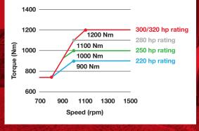
The B4.5 and B6.7 rapidly deliver high levels of torque from low engine speed to enhance vehicle driveability.
