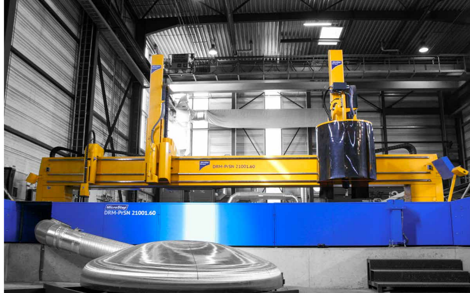
DRM machine for cutting of tank ends up to Ø 5,500 mm
