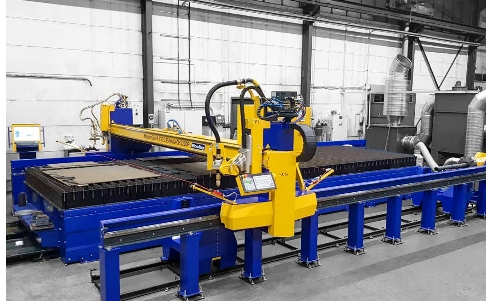
MasterCut with linear guidelines in the X-axis and a channel for pipe processing
