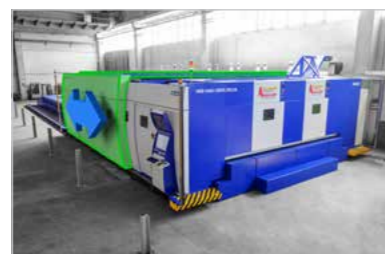
Mobile and retractable safety cabin
