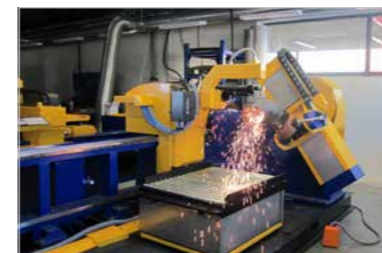
ElbowCut: Weld edge preparation on pipe elbows
