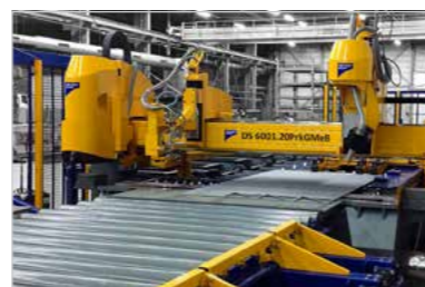
Automated processing of flat materials for steel structures
