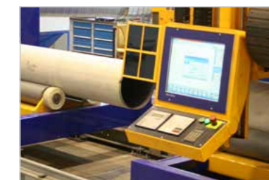
Operator terminal on the gantry
