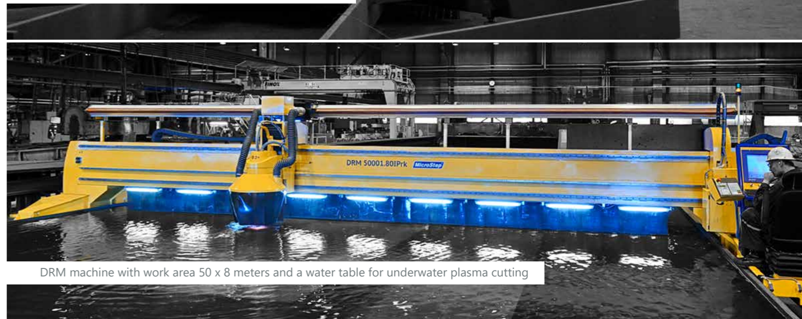
DRM machine for cutting of tank ends up to Ø 5,500 mm
