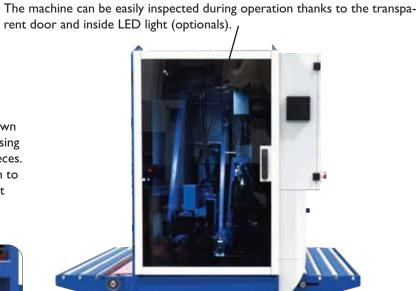
Infeed and outfeed table extensions to make easier the loading-unloading of workpieces.
