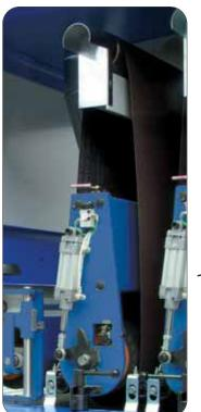
Cylinder unit equipped with 6 position Grit-set selector, revolver-type, for easily switching abrasive grit sequence, pneumatically activated.
