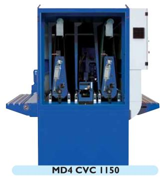
Deburring Polishing Machines with: **two** longitudinal abrasive belt working units and, **one** multifunction unit with vertical brushes.
