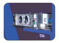
Sanding belt tracking photocell controlled.
