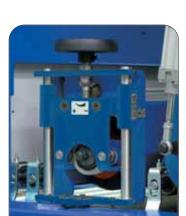
Longitudinal brush unit Ø 180 mm with manual height adjustment and mechanical thickness read-out. Lateral oscillation system of brush. Our brusches are available in various materials: steel, stainless steel, scotch brite and many others.
