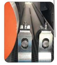
Double pressure rollers with micrometric precision adjustment mounted in front and rear of each working unit. Each working unit motor is equipped with disk brake allowing the machine to stop in a few seconds in case of emergency.
