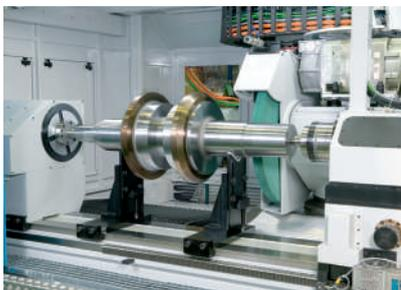
Automatic rotary axis, which enable the usage of several heads and the different machining operations with a single clamping.
