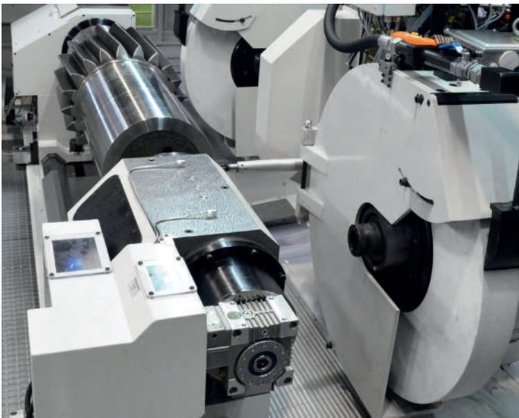
It is a grinding machine with 2 wheel heads, one for rough grinding and the other for finishing. It is designed for long cylindrical parts and it reduces dramatically the grinding cycle span.
