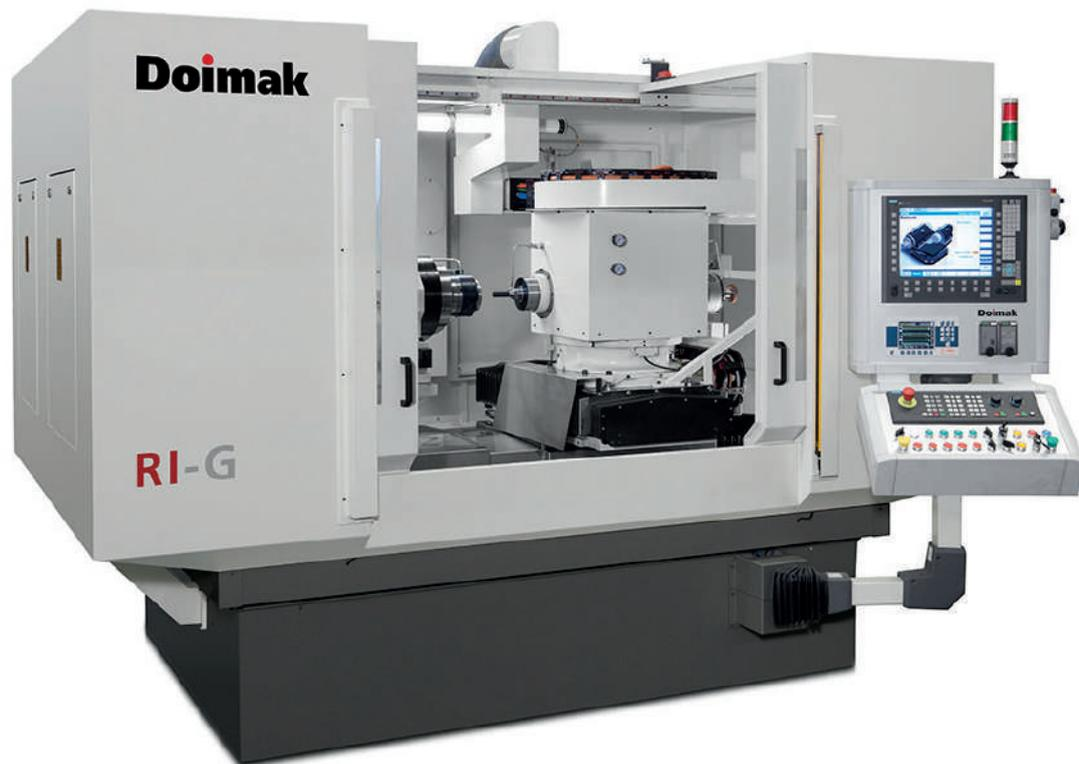
Doimak RI-G is designed for the internal grinding of the differential housing flange for rear axle.
